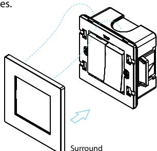
2. To install the surround, align surround locking clip onto the baseplate and press firmly on the surround until you hear a clear "click" sound.
