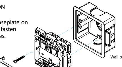
2. To install the surround, align surround locking clip onto the baseplate and press firmly on the surround until you hear a clear "click" sound.
