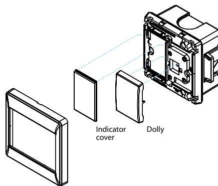
2. To install dolly and indicator cover, align dolly locking pin onto dolly base and press firmly the dolly. Align indicator cover locking pin onto indicator locking part and press firmly the indicator cover.
