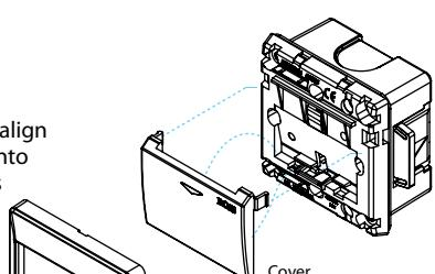
3. Align cover locking clip onto locking area and press firmly the cover until you hear a clear "click" sound.
