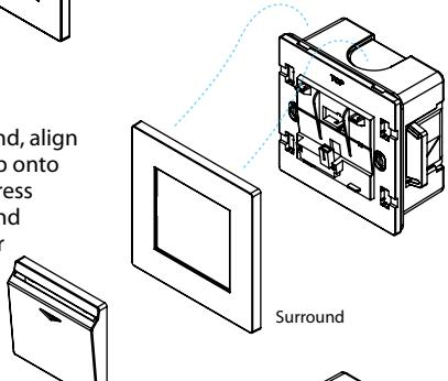
3. Align cover locking clip onto locking area and press firmly the cover until you hear a clear "click" sound.
