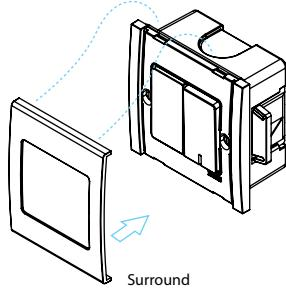
2. To install the surround, align surround locking clip onto the baseplate and press firmly on the surround until you hear a clear "click" sound.
