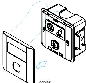
2. To install the cover, align cover locking clip onto the baseplate and press firmly on the cover until you hear a clear "click" sound.
