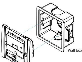
2. To install the surround, align surround locking clip onto the baseplate and press firmly on the surround until you hear a clear "click" sound.
