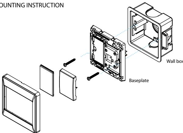
1. Align and place the baseplate on the wall box and then fasten the screw on both sides.
