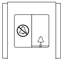
Bell Push Switch with "Do Not Disturb" Indicator.
