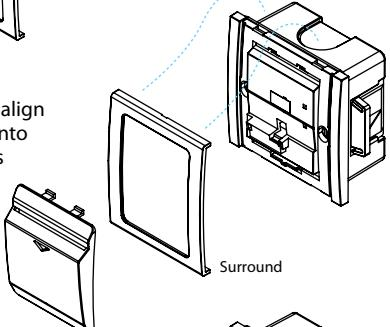
3. Align cover locking clip onto locking area and press firmly the cover until you hear a clear "click" sound.
