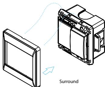
3. To install the surround, align surround locking clip onto the baseplate and press firmly on the surround until you hear a clear "click" sound.
